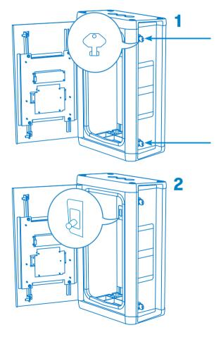
(\*) Tamper Switch: The Charge Point has a security switch (antitamper protection) installed that will avoid any charging session if the doors are opened.
