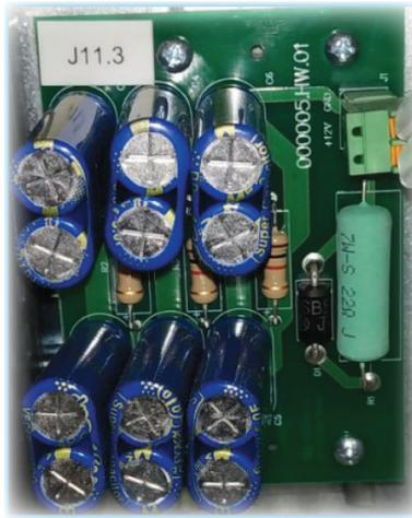
This board allows that the 12Vdc electronics remain supplied for few seconds when unit is powered OFF.
