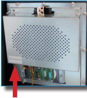
*The Ethernet port of the Master Charge Point is located at the bottom left side of the rear part of the HMI screen.*
