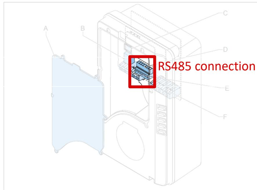
RS485 connection for Modbus RTU
