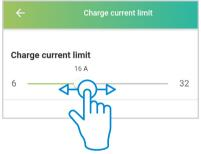
The modification of the supply current value will display a security message. The increase of this value can lead to electrical risks.
