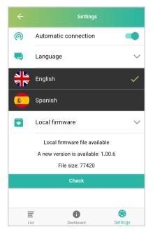
**Automatic connection:** This option allows the smartphone to directly pair to any Charge Point from the 'List' menu that is available. This option should be enabled to allow the Presence Recognition.
