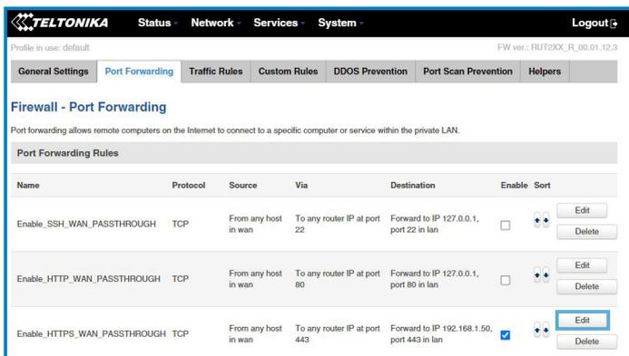
Once in Edit screen, insert 192.168.1.50 in "Internal IP address" field and click Save button.
