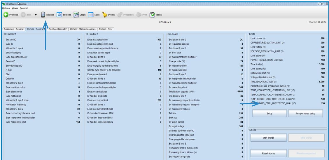
7- The pop-up window below appears, at **'Limit Power'** tab it is possible to set the maximum DC power output, it can be selected from 10kW until 150kW for CCS.
