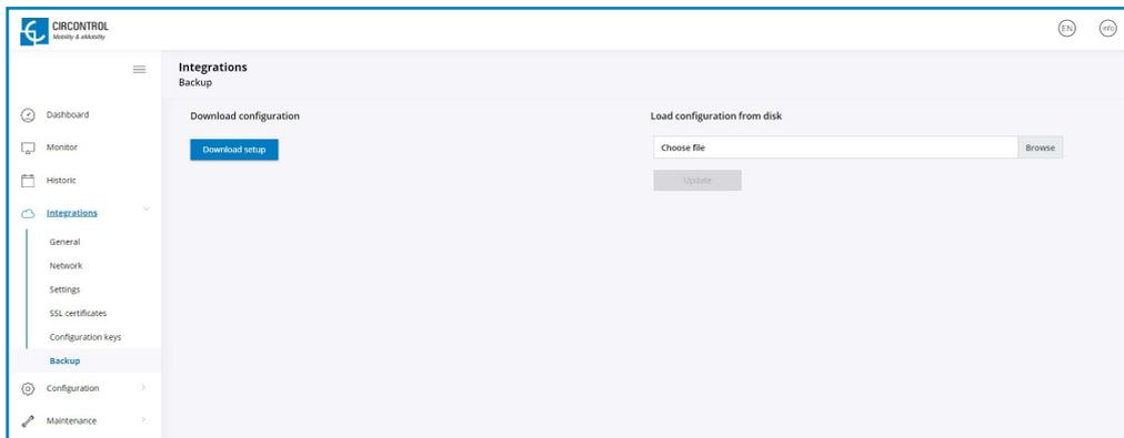
It is possible to download a backup of the Charge Point pressing 'Download setup' button. On the other hand, it can also be uploaded a backup previously downloaded from another Charge Point.
