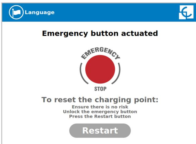
At first moment, the **'Restart'** touch button will be in light grey and it will not be able for pressing. Once emergency button has been unlocked, the **'Restart'** touch button will be in green and able to use.
