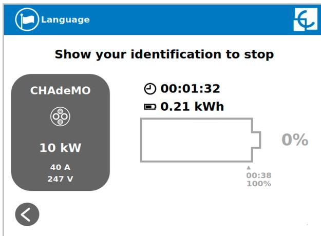
After showing the identification card, the Charge Point will allow you to stop the charging session by pressing over the ‘**Stop**’ touch button:
