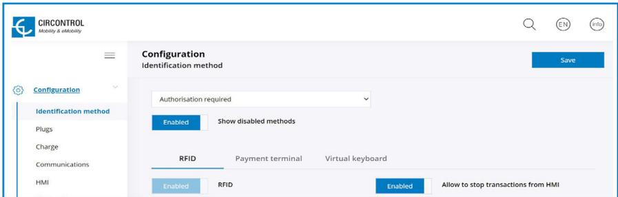
When the Charge Point includes payment terminal, it is necessary to enable the option to let the user pay with this method.
