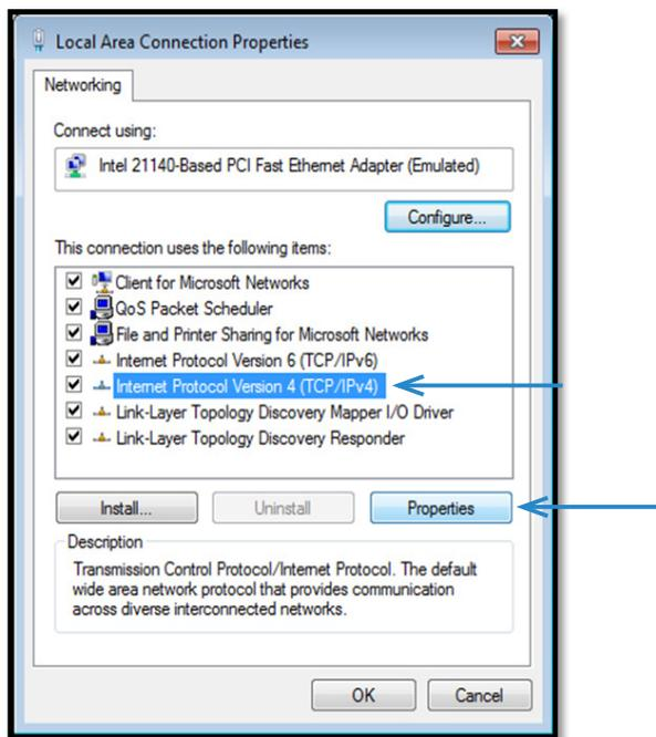
5- Setup IP address and subnet mask like as shown here below and click 'OK' twice to complete the assigning IP address process to the computer.
