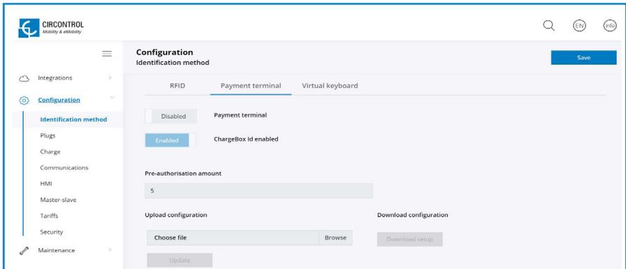
Enable ChargeBox Id option allows the system to differentiate every single charge point separately, in order to use this data by the back end system.
