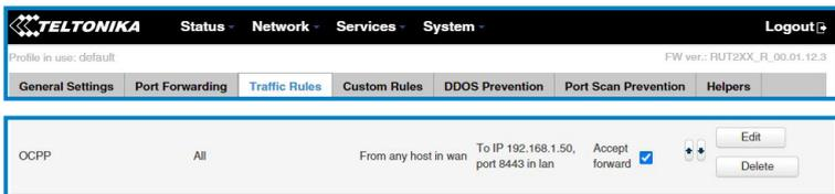
Check that the new line appears and tap enable check in case is disabled.
