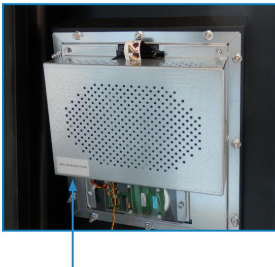
The Ethernet port is located at the bottom left side of the rear part of the HMI screen.
