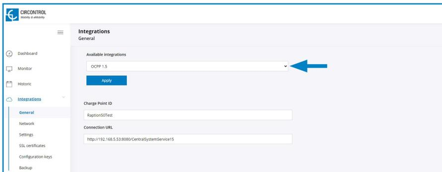
Charge Point supports different versions of OCPP but only one can be enabled at the same time.
