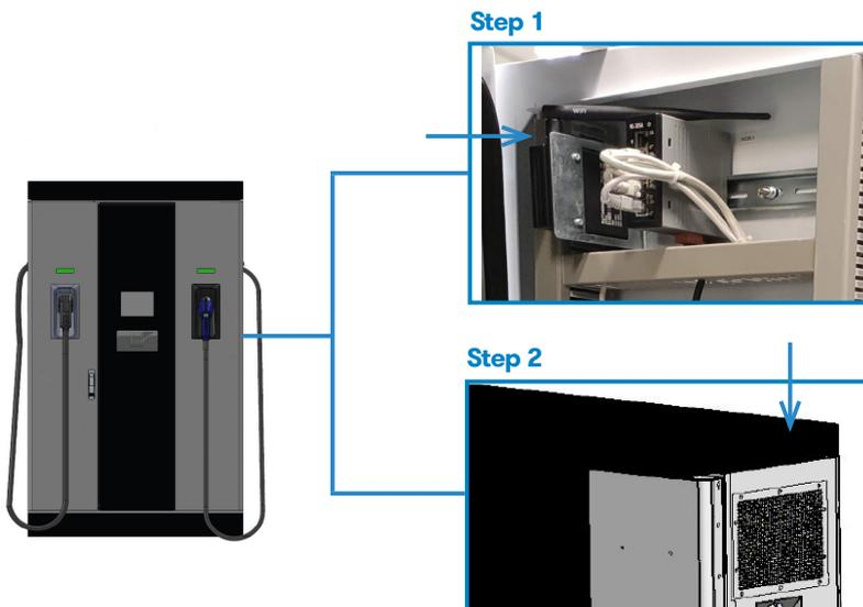
Step 1- Open Charge Point's right door and locate the modem, on the rear side.
