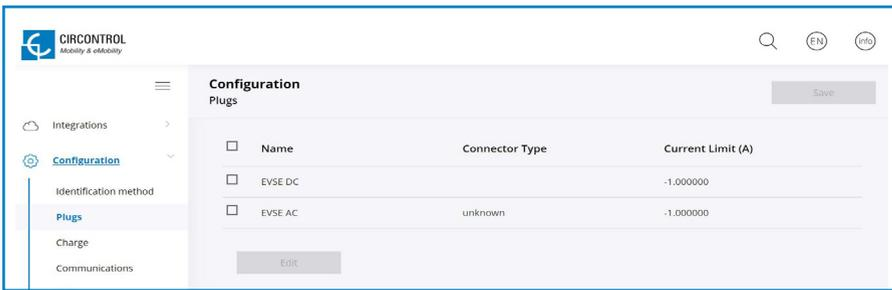
It is possible to enable and disable charging with quick charging (EVSE DC), slow charging (EVSE AC) or both in each Charge Point.
