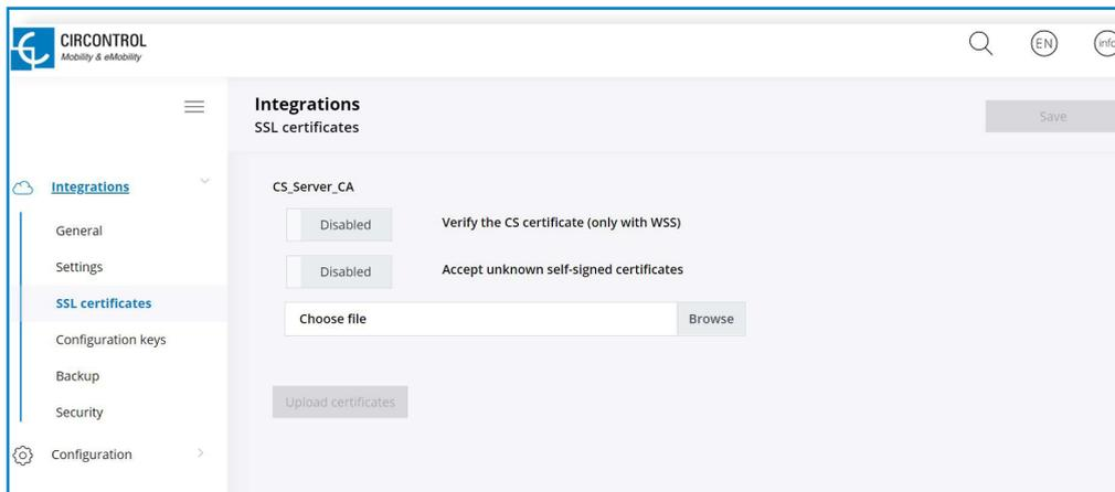
For WSS connections is needed a Central System certificate. Upload it in this section.
