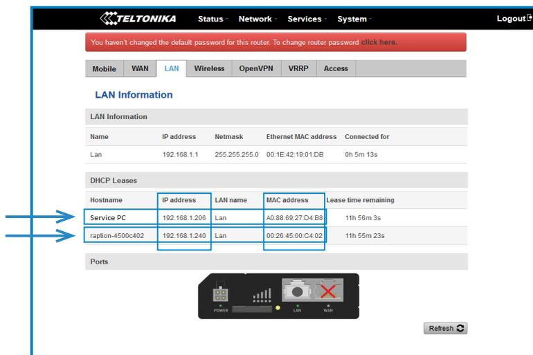
At 'DHCP Leases' check that the modem has detected the automatic IP address and MAC number for both, your Service PC and the Charge Point.
