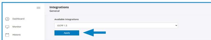
**NOTE:** Charge Point is working as stand-alone if **'none'** option is selected. All ID cards are authorized to start/stop a new charge transaction and no requests are sent to the backend.
