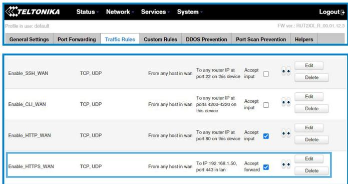
Once in Edit screen, insert 192.168.1.50 in "Destination address" field and 443 in "Destination port" field; then click Save button.
