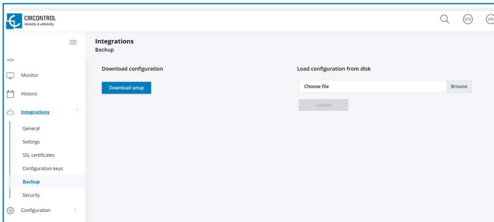
It is possible to download a backup of the Charge Point pressing 'Download setup' button. On the other hand, it can also be uploaded a backup previously downloaded from another Charge Point.
