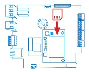
If the three LEDs are not on after inserting the SIM card, check the modem configuraton.
