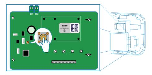
After that, the Charge Point will perform a system reboot and all the settings will be restored to factory values.
