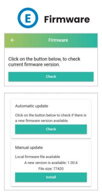
The Charge Point firmware can be upgraded through 'HiCharger' app. There are two different ways to perform the upgrade:
