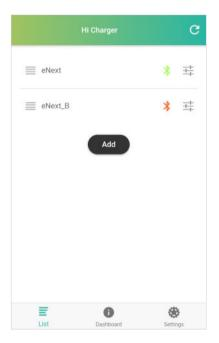
**'List'** view is an overview screen that shows the Charge Points that have been paired with the smartphone trough 'HiCharger' App. The connection status between the Charge Points and the smartphone is also shown and updated every 15 seconds.
