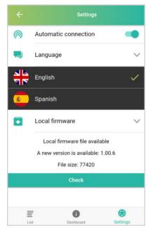
**Automatic connection:** This option allows the smartphone to directly pair to any Charge Point from the 'List' menu that is available. This option should be enabled to allow the Presence Recognition.
